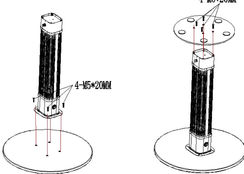
Step 1. Place table top bottom up on the ground, then align the four holes on the main body of the product to the four holes in the table top. Use a screwdriver to fix the main body of the product and the table top with 4 M5\*20MM screws. (e.g. Fig.1)
