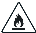
Caution: Risk of fire
